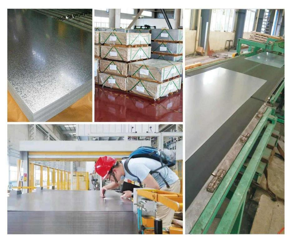
The thickness of the thinnest galvanized sheet is:  $0.12 \, \text{mm}$  Galvanized sheet thickness specifications:  $0.12 - 60 \, \text{mm}$  Galvanized sheet size specifications: Width:  $10 - 1500 \, \text{m}$
