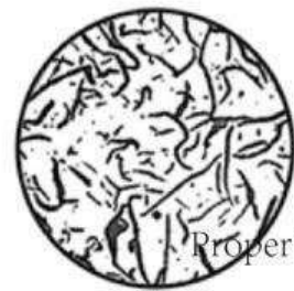
Gray Iron Excellent castability but "brittle"-less strength
